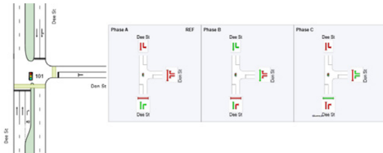
Figure 3.1 Dee St / Don St Traffic Signal layout and phasing
